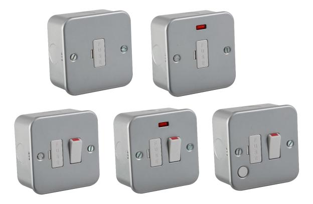
Fused spur units or connection units are an electrical switch with a built in fuse, designed for appliances that do not have or require a fused plug top. Fused spur units are also used for high powered electrical equipment with heavy continuous load, so that the appliance can be isolated by a single cable from a ring main for safety and maintenance purposes. 13A rated available with and without a double pole switch/neon.
