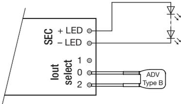
**300 mA:** Terminal 0 and 1 connected with 0 Ω wire (max. 6 cm length) or resistor ADV Plug Type A BR (article number: 28001771)
