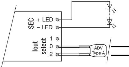
**275 mA:** Terminal 0 and 2 connected with resistor ADV Plug Type B BR (article number: 28001772)
