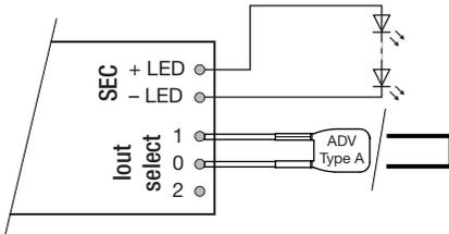
**325 mA:** Terminal 0 and 2 connected with resistor ADV Plug Type C BR (article number: 28001773)
