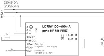
The voltage line for switchDIM / corridorFUNCTION must be the same line as on the mains input of the Driver. In switchDIM applications the DALI interface as well as the integrated DALI bus power supply (IPS) can not be used.
